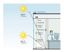
Peak solar altitudes during the year on the south elevation, 40° north latitude. SolarTrac system preset to five or more positions plus user-defined solar penetration (3 ft./91cm shown here).
